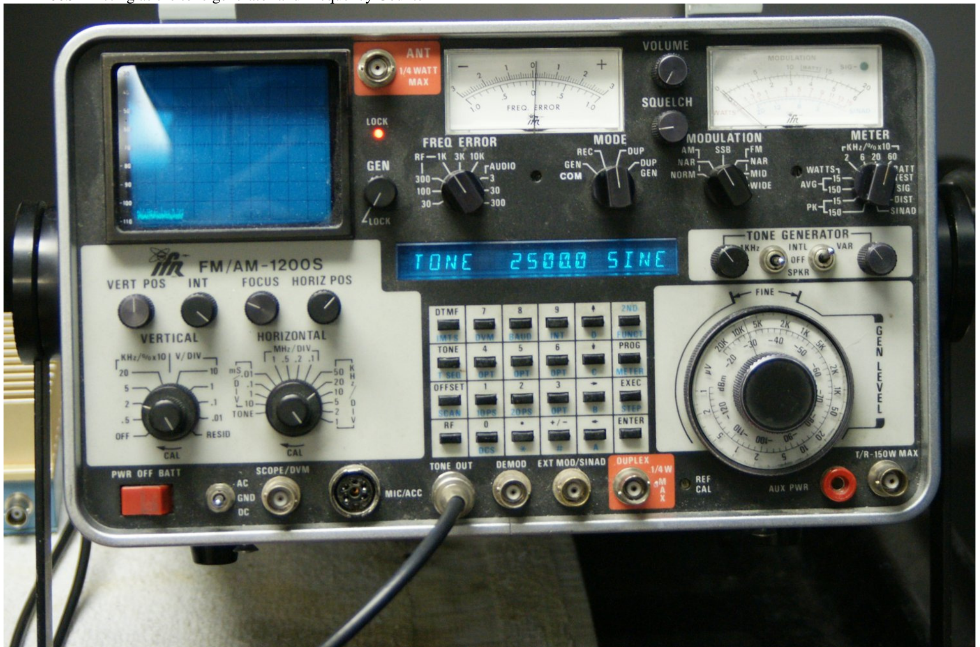
IFR 1200S – Acting as the tone generator and Frequency Counter
