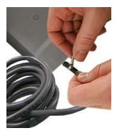
4. Beginning over the installed electrical tape, twist the Itron cable armor onto the 500W ERT Module cable using a right-handed twist.
