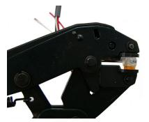
3. Squeeze the handles to crimp the connector. Apply pressure until the cap is fully seated (at least three seconds).
