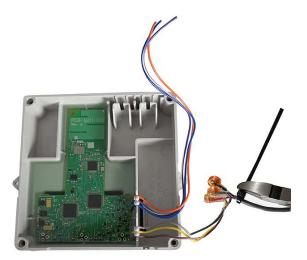
7. Place the cable connection into the 500W ERT Module housing with the cable ties to the inside.
