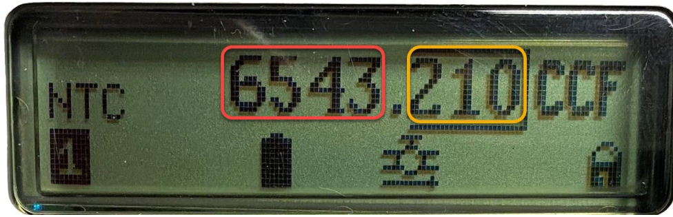
Figure 2 Intelis Gas Meter configurable display
