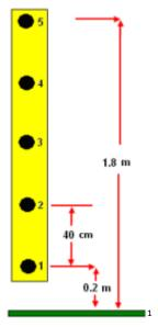
The following diagram is an example of the setup used for most tests, excluding magnetically mounted vehicle antennas.
