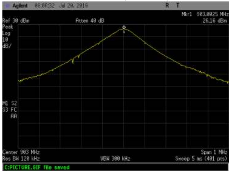
Channel 1 of 120 903.0 MHz AM OOK power level 3, +27dbm nominal
