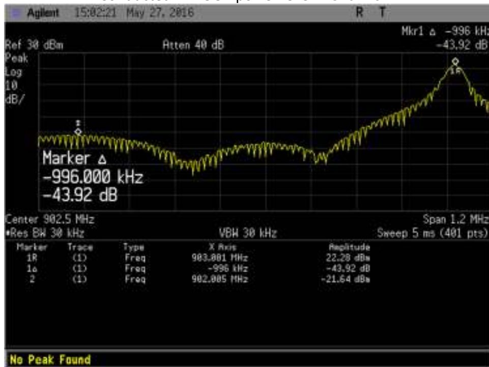
Conducted AM OOK power level 2 Channel 1
