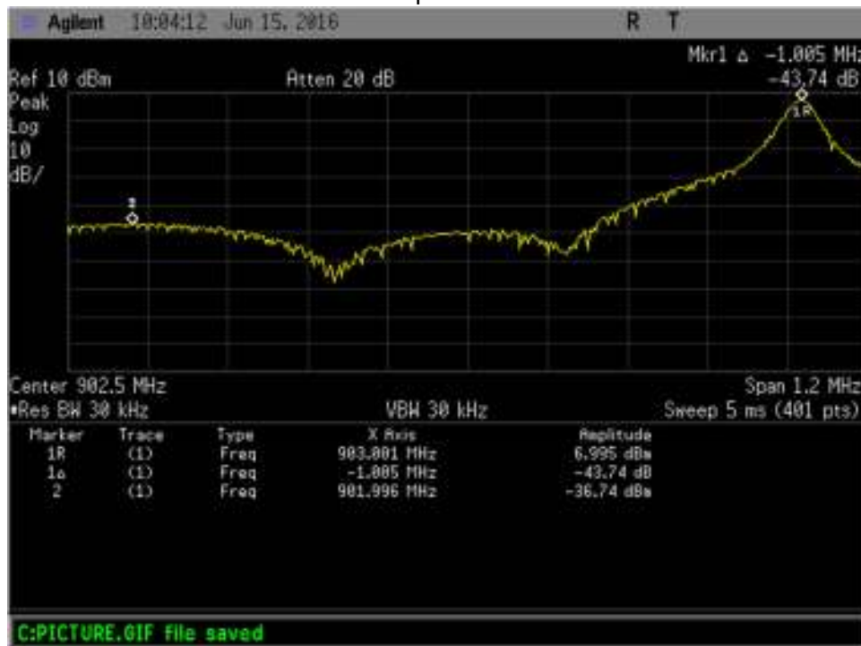
Conducted AM OOK power level 1 Channel 1
