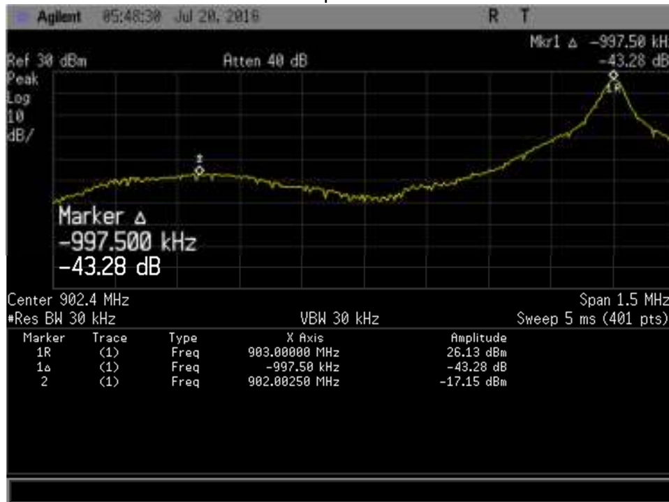
Conducted AM OOK power level 3 Channel 1
