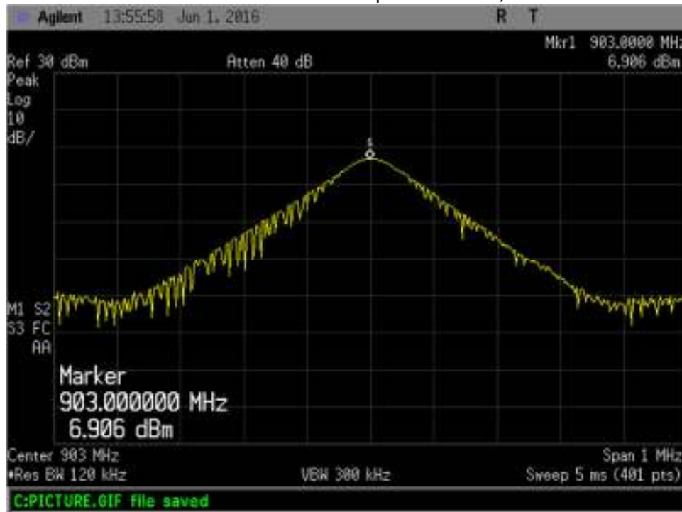
Channel 1 of 120 903.0 MHz AM OOK power level 1, +10dbm nominal
