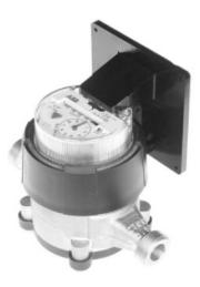
1. Push the hollow pin (1) completely out of its location and separate the Cellular 500W remote module mounting bracket (2) from the meter register collar (3).
