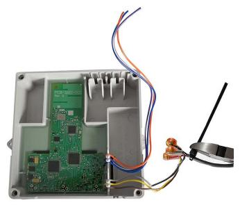
6. Place the cable connection into the Cellular 500W remote module housing with the cable ties to the inside.
