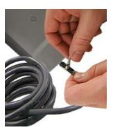
4. Beginning over the installed electrical tape, twist the Itron cable armor onto the Cellular 500W remote module cable using a right-handed twist.
