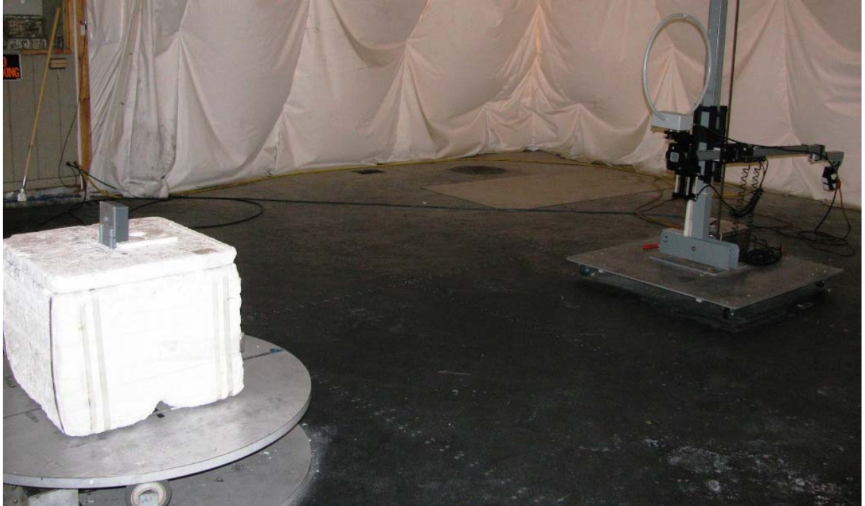
Photo 3: Test setup for radiated spurious between 9kHz and 30MHz with Loop Antenna shown and Range Extender.
