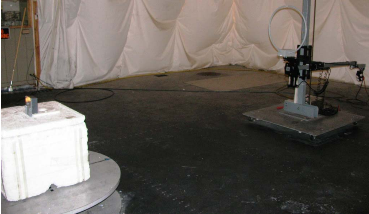
Photo 2: Test setup for radiated spurious between 9kHz and 30MHz with Loop Antenna shown and Range Extender.
