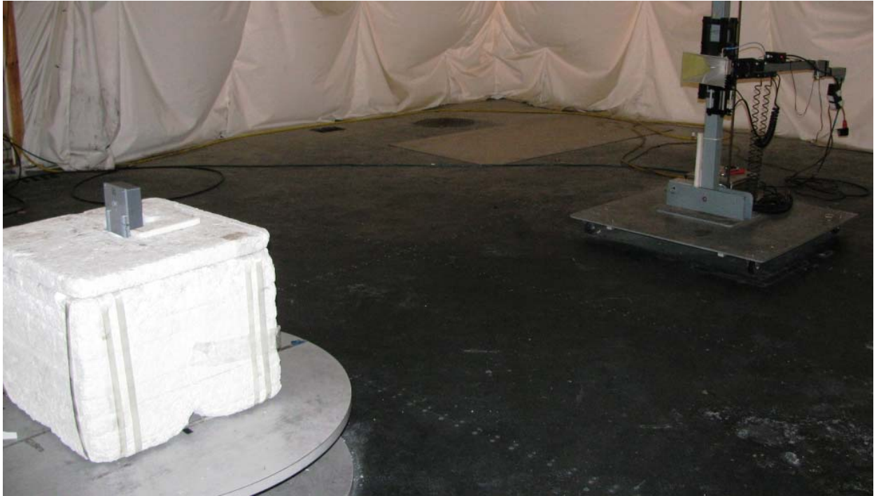
Photo 15: Test setup for radiated spurious emissions below 18GHz with horn antenna in vertical polarity and Range Extender.
