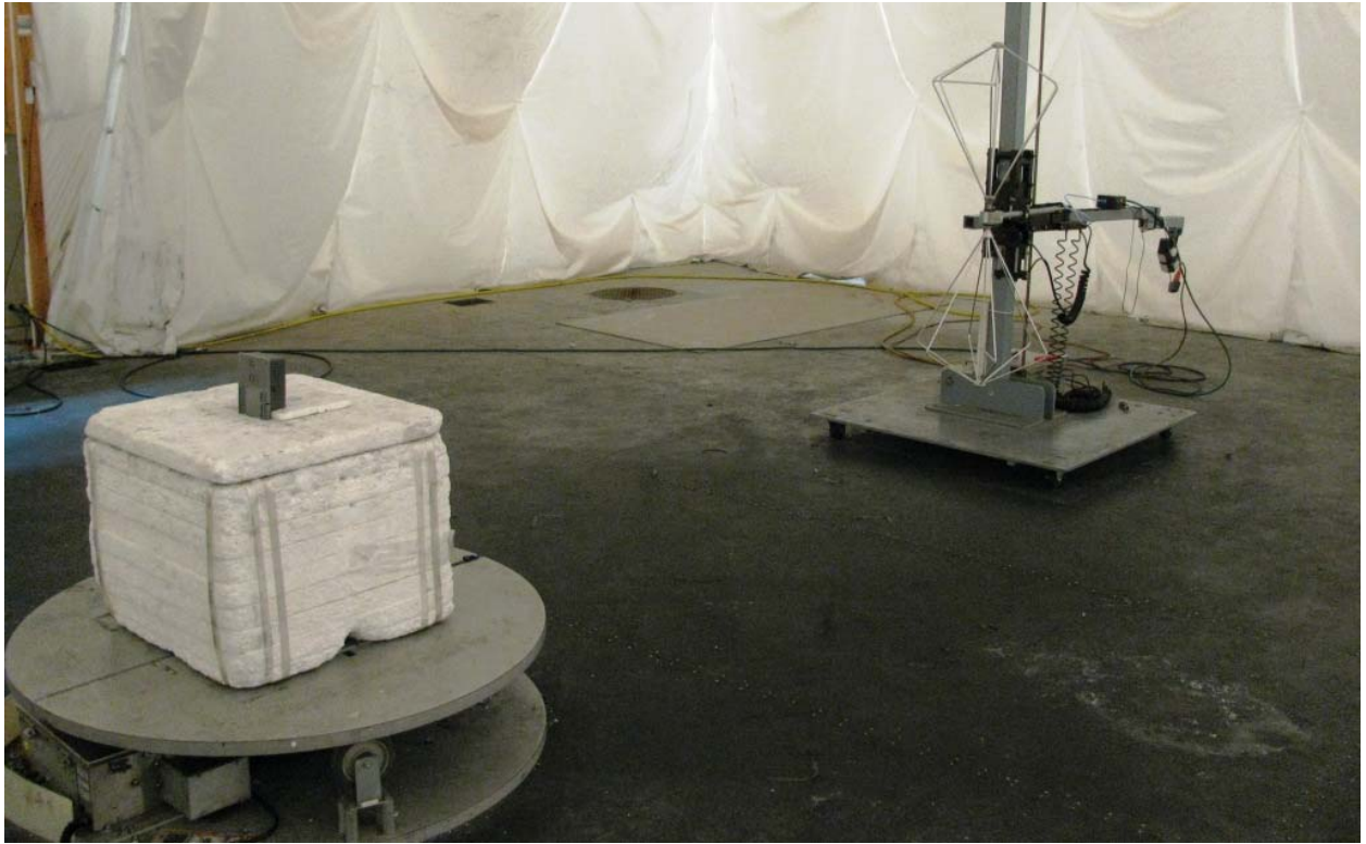
Photo 7: Test Setup for Radiated Spurious measurements between 30MHz and 300MHz using Biconical antenna shown here in vertical orientation and Range Extender.
