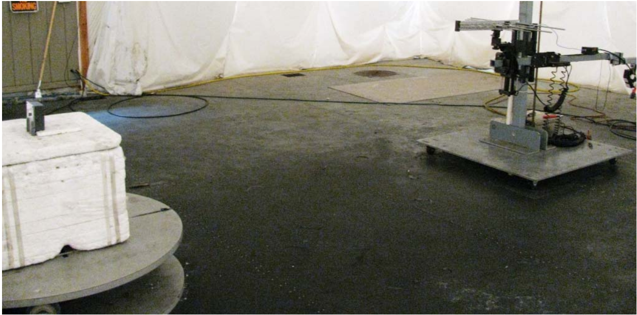
Photo 9: Test setup for RX radiated spurious between 200MHz and 2GHz with Log Periodic in horizontal orientation shown with Range Extender.
