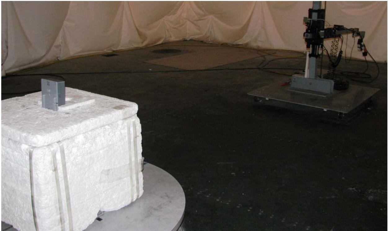
Photo 19: Test setup for radiated spurious emissions above 18GHz (horizontal polarity) shown with Range Extender.
