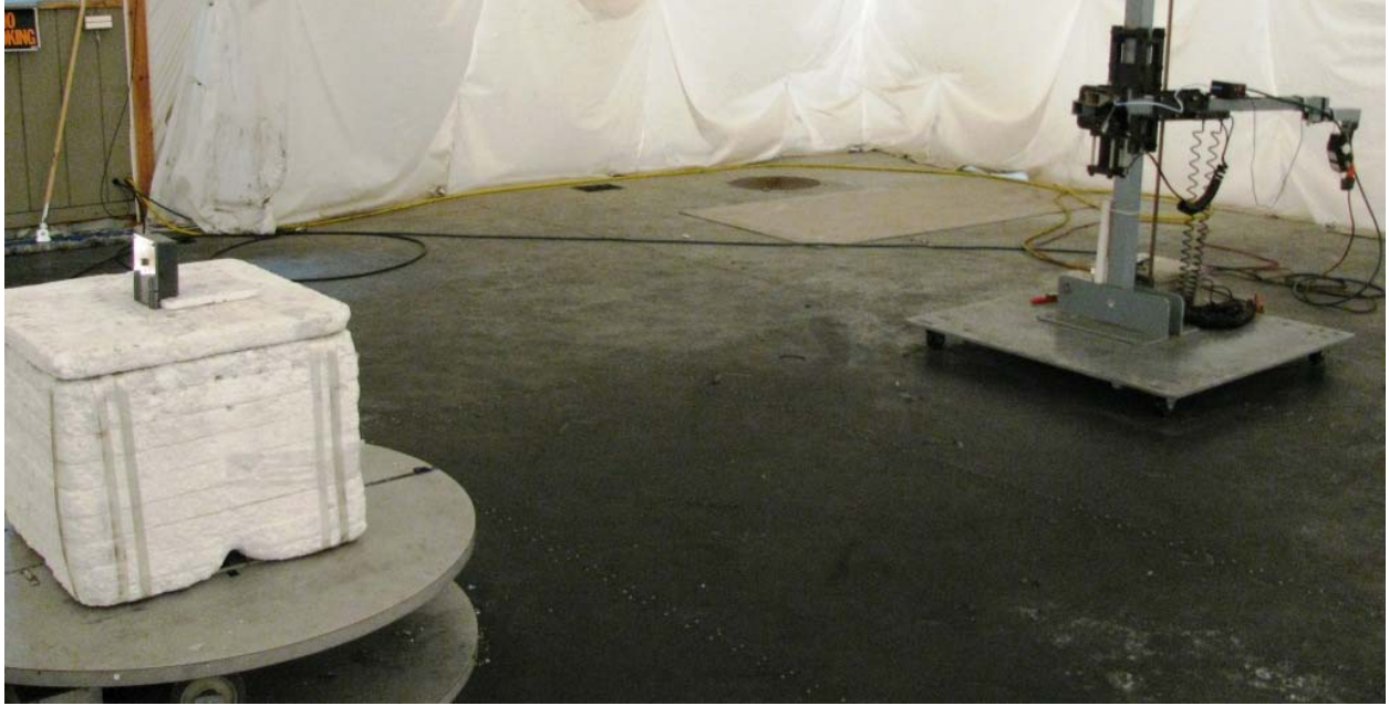
Photo 20: Test setup for radiated spurious emissions above 18GHz (vertical polarity) shown with Range Extender.
