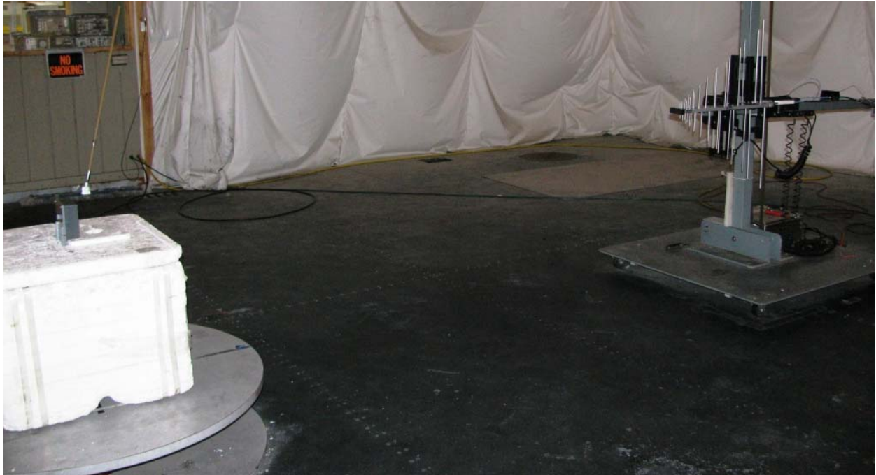
Photo 10: Test setup for TX radiated spurious between 200MHz and 2GHz with Log Periodic in vertical orientation shown with Range Extender.
