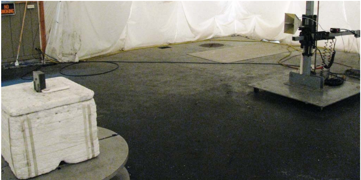
Photo 14: Test setup for radiated spurious emissions below 18GHz with horn in horizontal polarity and Range Extender.
