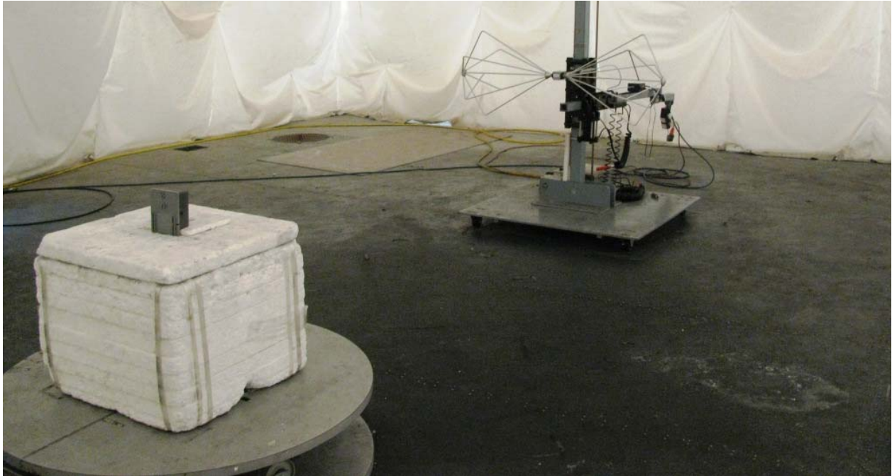
Photo 6: Test Setup for Radiated Spurious measurements between 30MHz and 300MHz using Biconical antenna shown here in horizontal orientation and Range Extender.
