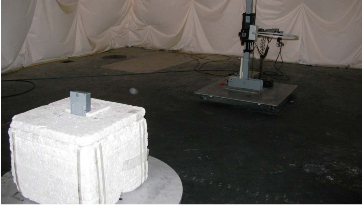
Photo 4: Test setup for radiated spurious between 9kHz and 30MHz with Loop Antenna and Range Extender.
