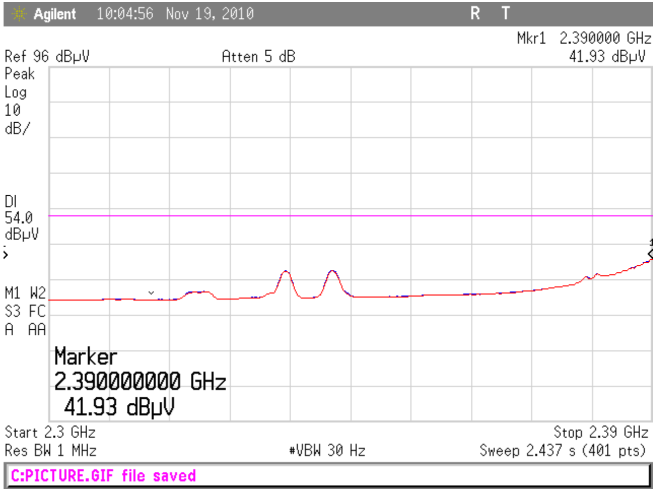
Figure 22: Average Vertical Radiated Band Edge (2405MHz Fundamental)
