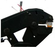
3. Crimp the connector by squeezing the handles until the connector cap is fully seated. Continue to apply pressure for three seconds.
