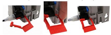
**Note** For future meter or ERT module servicing, break the security seal by pulling the seal apart. The original protective connector covers can be reused if kept clean and dry. Install a new security seal after servicing either device. To order replacement security seals, see the *Water ERT Module Ordering Guide* (PUB-0063-001).
