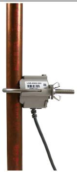
4. Insert the mounting plate over the U-bolt's threaded screw ends. Attach the two wing nuts over the clamp screw ends and tighten the wing nuts until snug (to a minimum of 5-inch pounds) to prevent device rotation on the pipe. After you tighten the second wing nut, check the Leak Sensor to verify the device is snug. If the sensor moves, tighten the wing nuts until there is no movement.
