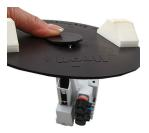
3. Slide the adapter assembly into the pit lid with the foam spacers positioned on each side of the pit lid slot.
