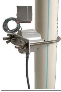
**Caution** Do not tighten the Leak Sensor to more than 20 inch-pounds. Over-tightening could damage the Leak Sensor housing and/or the pipe.
