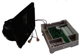
5. Place the ERT module on the register, ensuring the edge of the ERT module housing is seated properly around the perimeter of the register as shown below.
