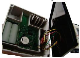
3. To wire the 100WP-R/100WP-R+ to the RTR 2-wire register, connect the ERT module wires to the 2-wire register using gel-cap connectors (see Using Gel cap Connectors). After connecting the wires, carefully tuck the connectors into the ERT module housing.
