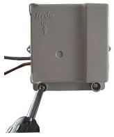
6. Insert a tamper seal over each mounting screw and drive into place with a nut driver or a similar tool.
