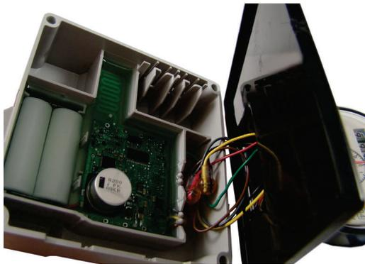
3. To wire the 100WP-R/100WP-R+ to the RTR 2-wire register, connect the ERT module wires to the 2-wire register using gel-cap connectors (see [Using Gel cap Connectors](#)). After connecting the wires, carefully tuck the connectors into the ERT module housing.
