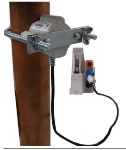
**Caution** Do not tighten the Leak Sensor to more than 20 inch-pounds. Over-tightening could damage the Leak Sensor housing and/or the pipe.
