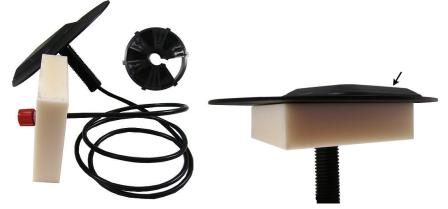
2. Insert the antenna connector through the rectangular opening in the threaded collar.
