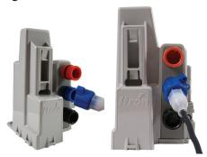
4. Rotate the connector locking ring until the security holes align.
