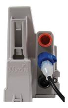
Caution Do not force the connector ends together. While you hold the LS connector, engage the ERT module's connector by rotating the locking ring until both connectors securely connect. Twist only the connector locking ring, not the body of the connector. Twisting the connector body could damage the connector's pins.
