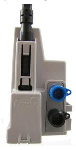
2. Push the antenna coupler into the antenna slot until the coupler locks into the tabs of the antenna slot.
