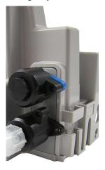
3. Twist the register cable's black coupling nut to align the two tabs.
