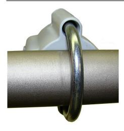
4. Insert the mounting plate over the U-bolt's threaded screw ends. Attach the two wing nuts over the clamp screw ends and tighten the wing nuts until snug (to a minimum of 5-inch pounds) to prevent device rotation on the pipe. After you tighten the second wing nut, check the Leak Sensor to verify the device is snug. If the sensor moves, tighten the wing nuts until there is no movement.
