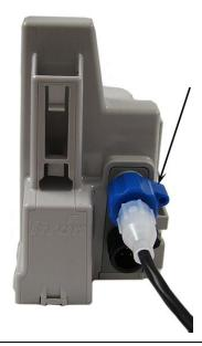
**Caution** Do not force the connector ends together. While holding the LS connector, engage the 100W connector by rotating the locking ring until both connectors securely connect. Twist only the connector locking ring, not the body of the connector. Twisting the connector body could damage the connector's pins.
