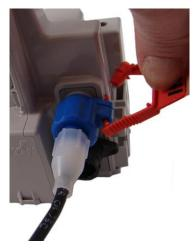
2. Insert the pointed end of the security seal into the capped end and push until the seal locks.
