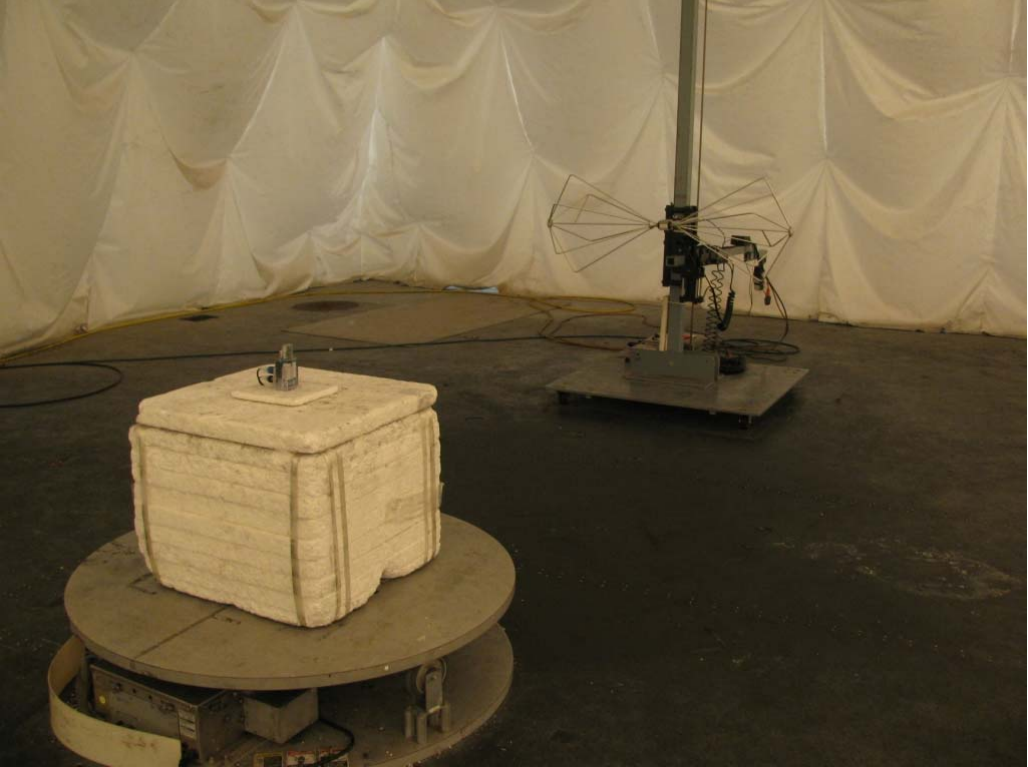
100WA test setup photos; EWQ100WA and 864D-100WA
