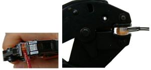
Note Do not strip lead wire prior to inserting the wire into the gel connector.
