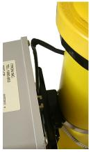
14. Insert the mounting screws and tighten in an alternating pattern.
