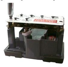
9. Slide the endpoint cover over the index and housing. The endpoint label should be clearly visible and easily read.
