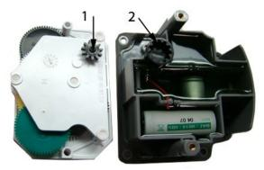
3. After the drive gear aligns with the wriggler gear, the mounting holes line up.
