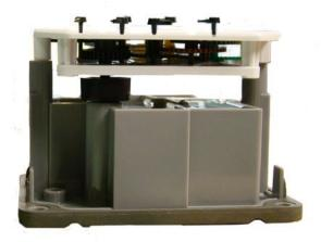
4. Using the original index mounting screw or a replacement screw (if necessary), place one 6 - 32 5/8" screw into the index's right mounting screw hole. Attach the screw to the endpoint housing's right-index mounting post just enough to hold the screw and the right end of the index in place. Install and tighten the left index mounting screw. Tighten the right index mounting screw completely. Install and tighten index mounting screws evenly.
