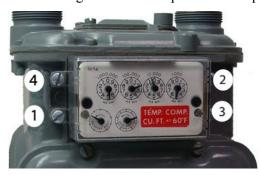
2. Examine the mounting screws. If they are 5/8" long and not corroded, keep them to re-attach the 100G Datalogging gas endpoint assembly. If the screws are not the correct length or if the screws are corroded, discard.
