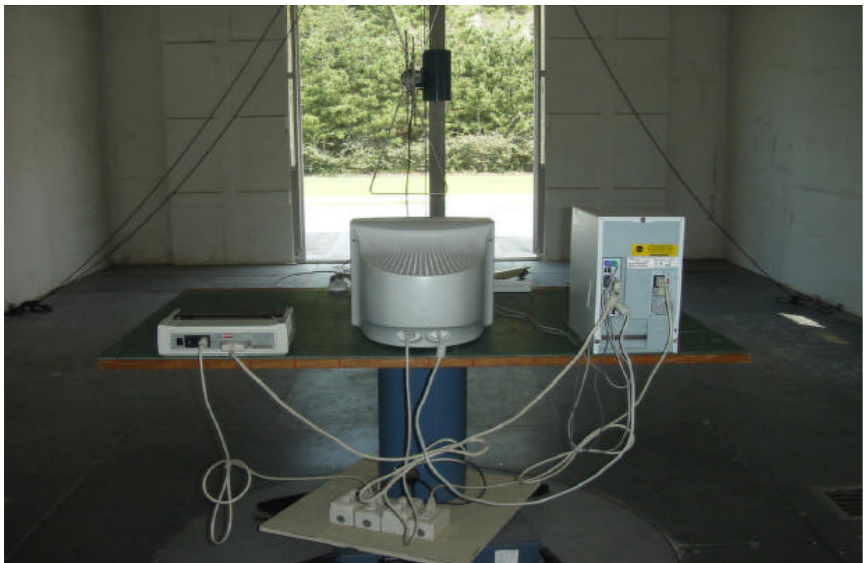
Radiated Emission 30MHz ~ 1000MHz
