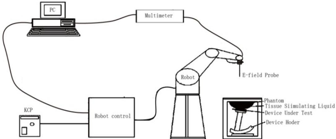
*Figure 1: Schematic diagram of the SAR measurement system*
