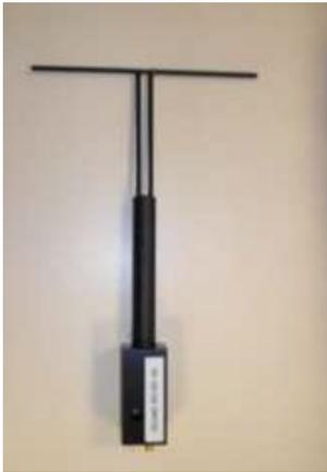
The dipoles used is based on the IEEE Std 1528, and is complied with mechanical and electrical specifications in line with the requirements of both FCC and KDB requirement.
