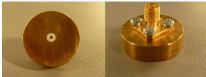
**Figure 1** – MVG LIMESAR Dielectric Probe
