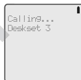
The screen displays **Calling:** and the name and extension number of the destination device. When the call is answered, the screen displays **Int.** and a timer.
