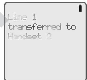
The screen displays **Line X transferred to XX** (**X** is the line number and **XX** is the device and extension number). The destination device rings.
