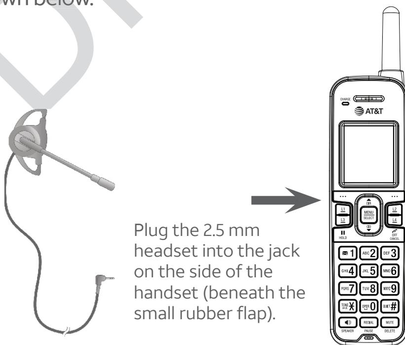
Plug the 2.5 mm headset into the jack on the side of the handset (beneath the small rubber flap).
