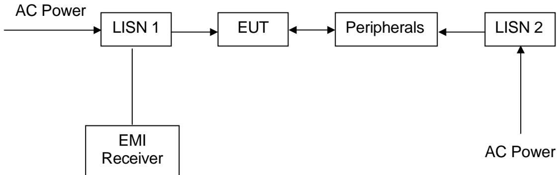
The EUT along with its peripherals were placed on a 1.0m(W)×1.5m(L) and 0.8m in height wooden table and the EUT was adjusted to maintain a 0.4 meter space from a vertical reference plane. The EUT was connected to power mains through a line impedance stabilization network (LISN), which provided 50 ohm coupling impedance for measuring instrument and the chassis ground was bounded to the horizontal ground plane of shielded room. The excess power cable between the EUT and the LISN was bundled.
