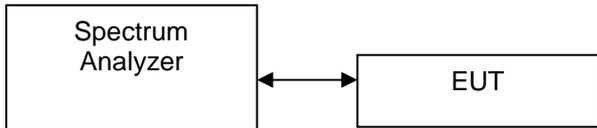
**4.1 Maximum Conducted (peak) Output Power at Antenna Terminals**
