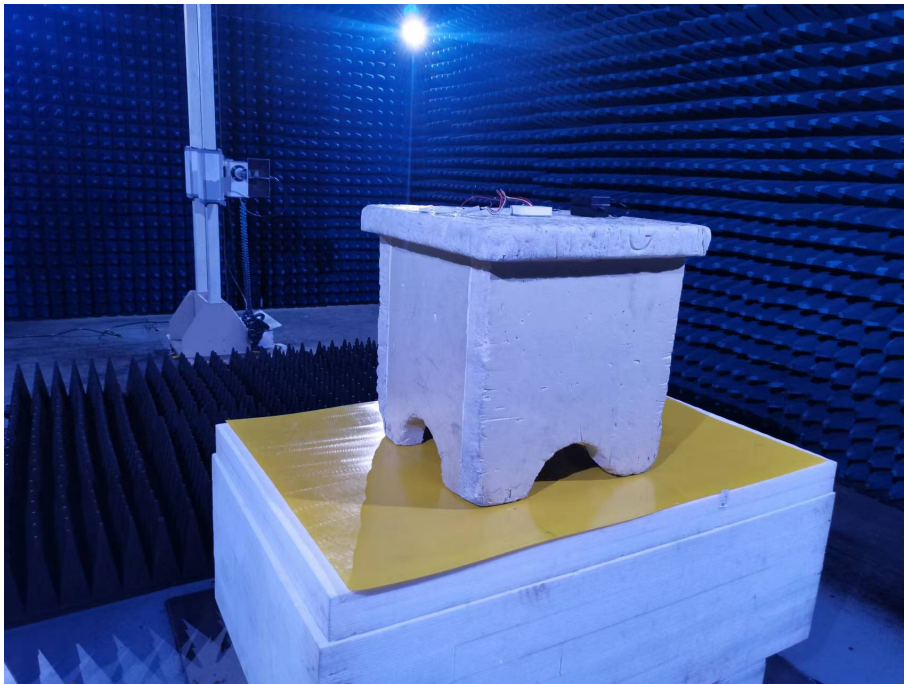
Photo of Radiated Emission Measurement (Above 1G)
