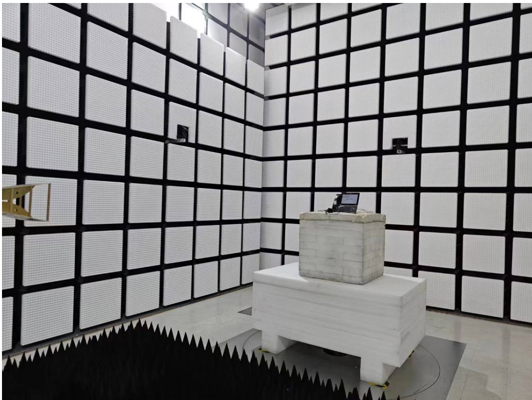
Radiated Emission Above 1GHz View
