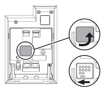
2. Slide the base power switch to the off position.
