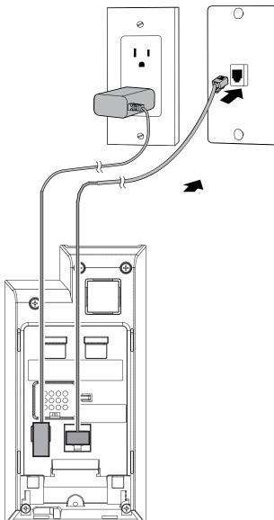
2. When the telephone base has been initially installed, make sure the power adapter is securely plugged into an outlet not controlled by a wall switch, and the Ethernet cable is plugged into the network wall jack.
