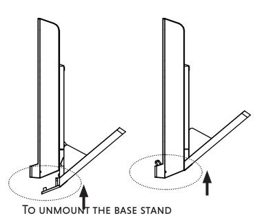
Simply slide the base stand down and lift it from the charger.
