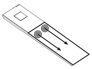
3. Lift the battery cover off the handset.
