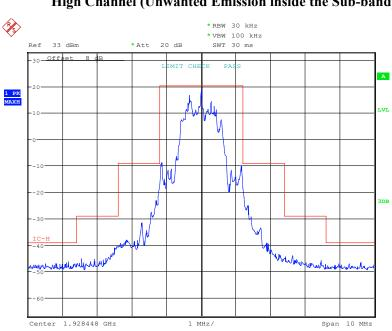
High Channel (Unwanted Emission inside the Sub-band)
