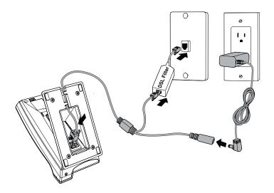
2. When the telephone base has been initially installed, make sure the power adapter is securely plugged into an outlet not controlled
