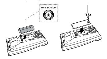
3. To replace the handset cover, align all the tabs on the base compartment battery cover against the corresponding grooves, then install the screw.
