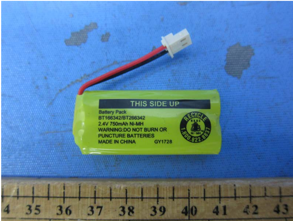
Figure 3 - 2.4V 750mAh Coslight Ni-MH rechargeable battery
