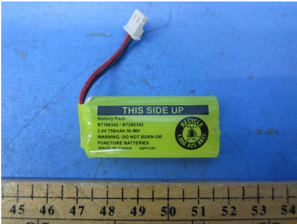
Figure 4 - 2.4V 750mAh GPI Ni-MH rechargeable battery
