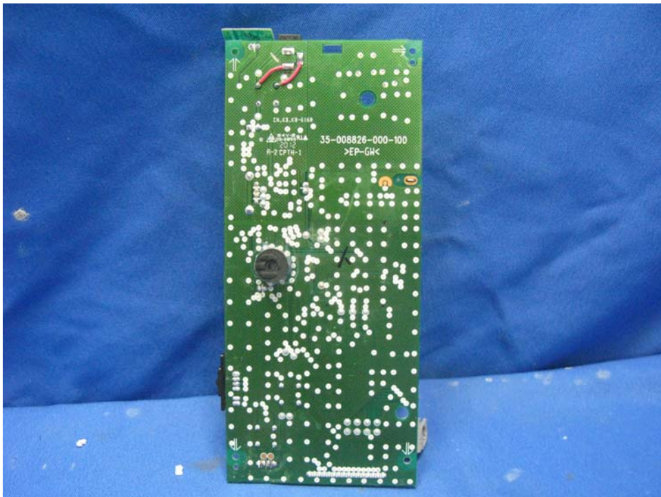
Deskset Main PCB solder side
