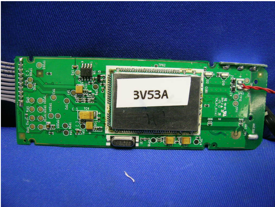
Handset Main PCB comp side
