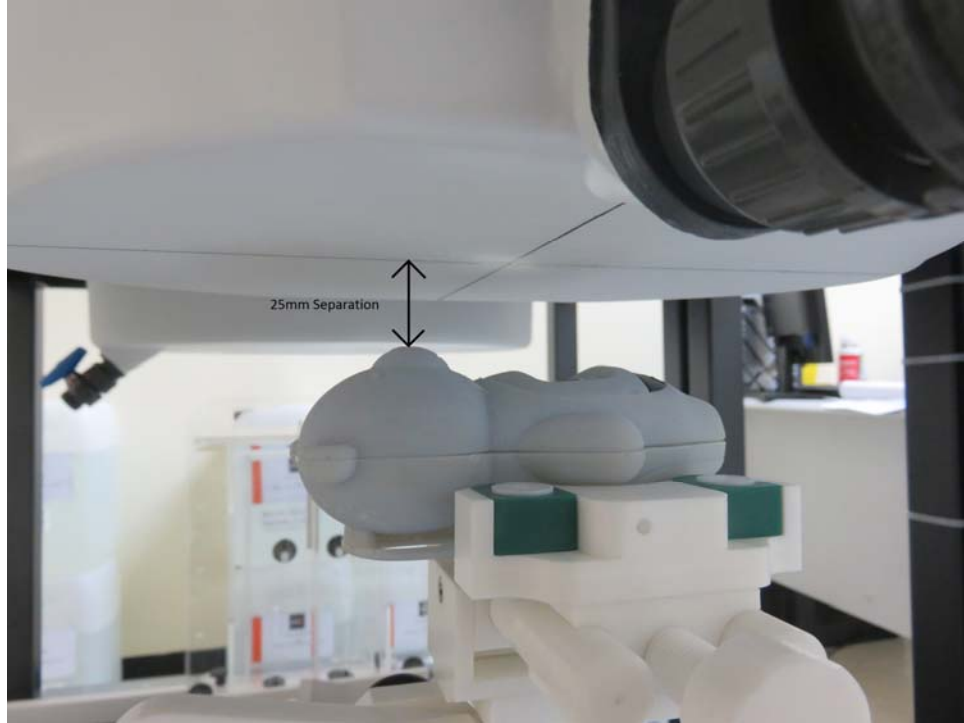
Figure 1 – Front surface with 25mm Separation
