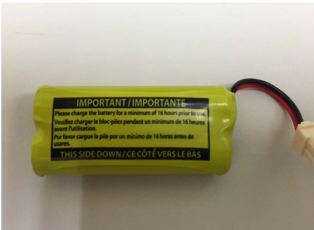
Figure 6 – 2.4V 750mAh Ni-MH Corun rechargeable battery back view
