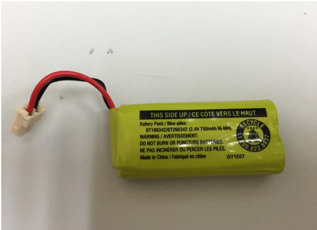
Figure 7 – 2.4V 750mAh Ni-MH Coslight rechargeable battery front view
