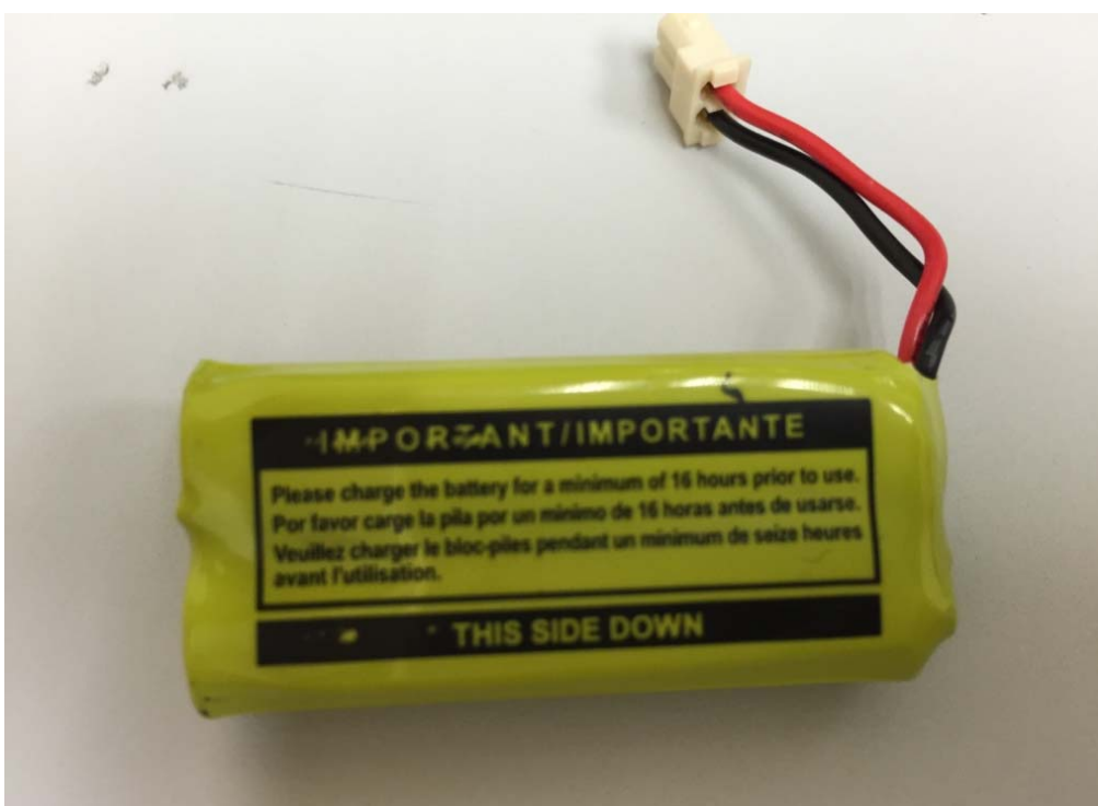
Figure 4 – 2.4V 750mAh Ni-MH GPI rechargeable battery back view
