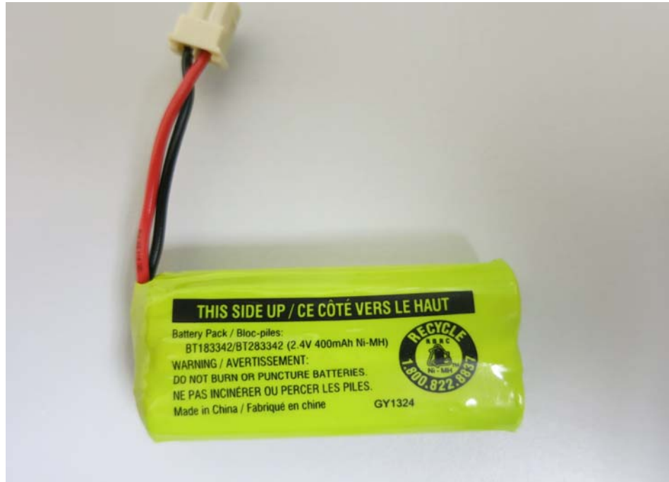
Figure 9 – 2.4V 400mAh Ni-MH Coslight rechargeable battery front view
