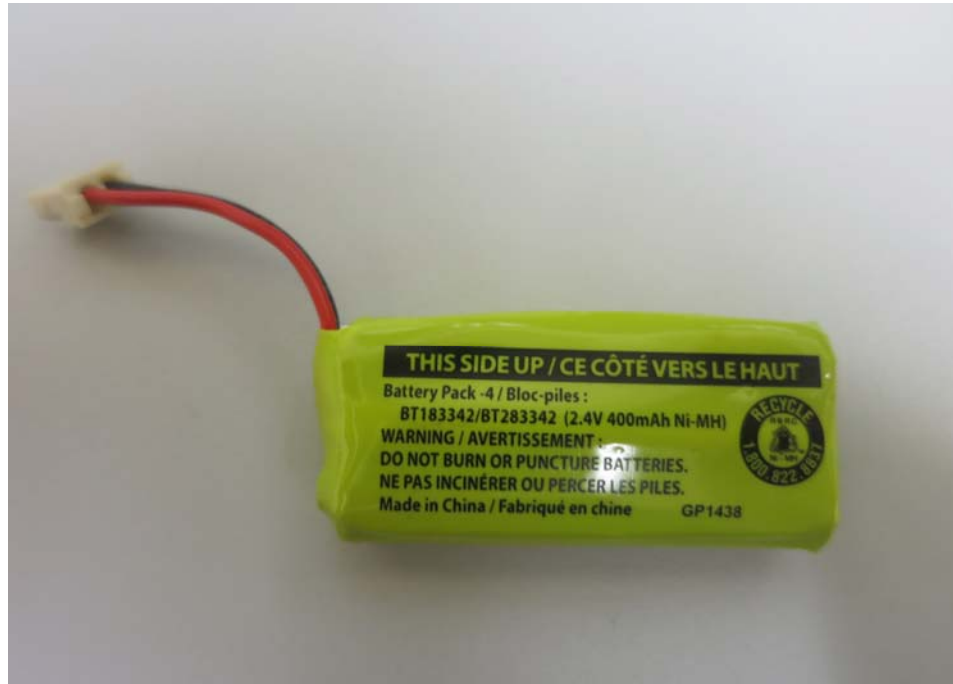
Figure 7 – 2.4V 400mAh Ni-MH GPI rechargeable battery front view
