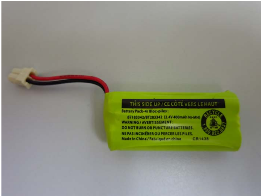
Figure 5 – 2.4V 400mAh Ni-MH Corun rechargeable battery front view
