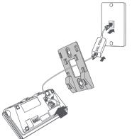
Align the holes on the wall-mount bracket with the standard wall plate and slide the wall-mount bracket down until it locks securely.
