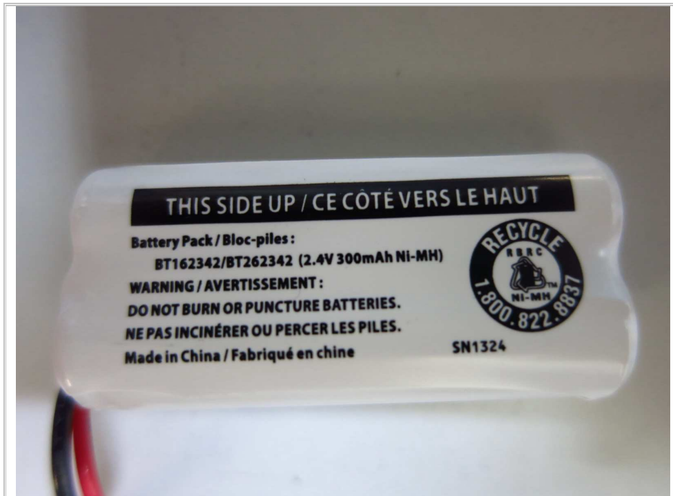
Figure 9 – 2.4V 300mAh Ni-MH Sanik rechargeable battery front view
