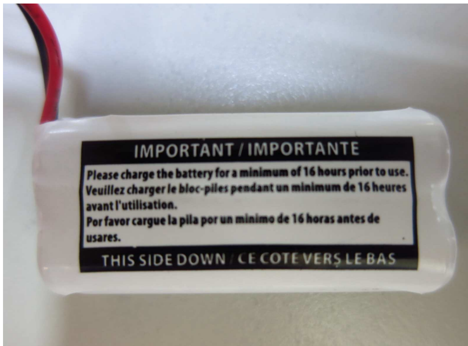
Figure 10 – 2.4V 300mAh Ni-MH Sanik rechargeable battery back view
