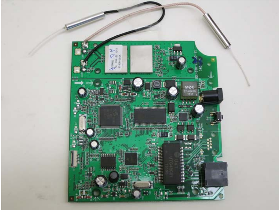
Base Unit Main PCB comp side with 2 antennas
