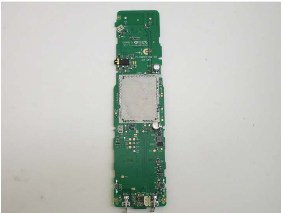
Handset Main PCB comp side (View 2)
