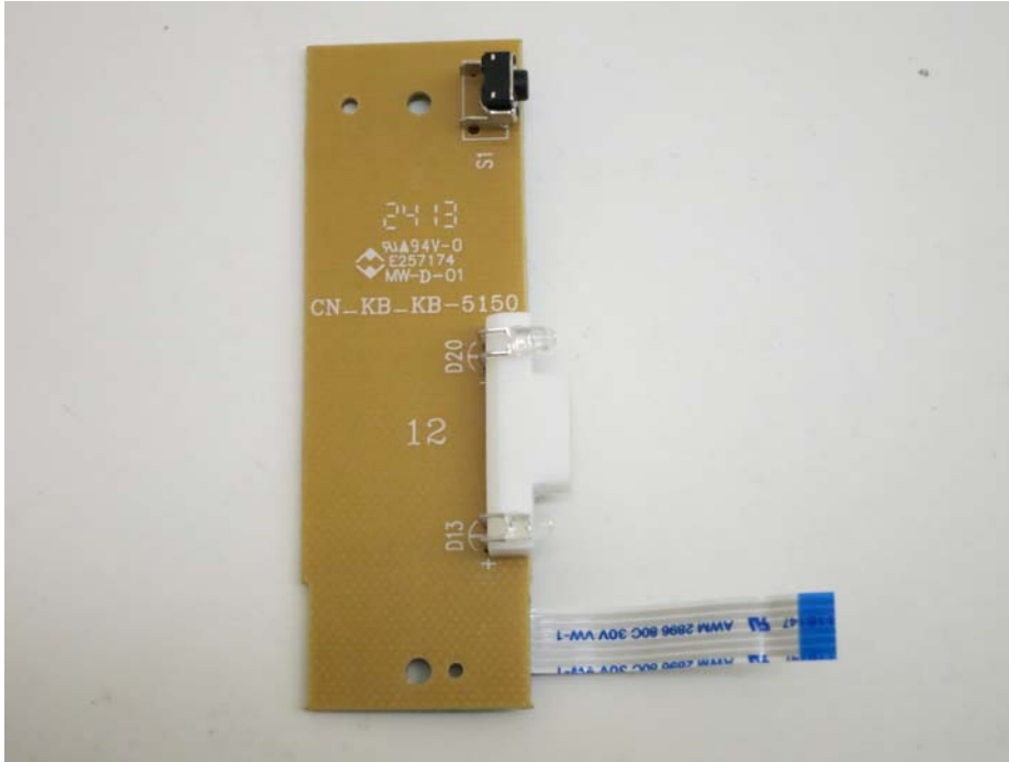
Base Unit Key PCB comp side
