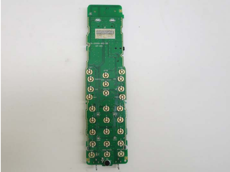
Handset Main Keypad side
