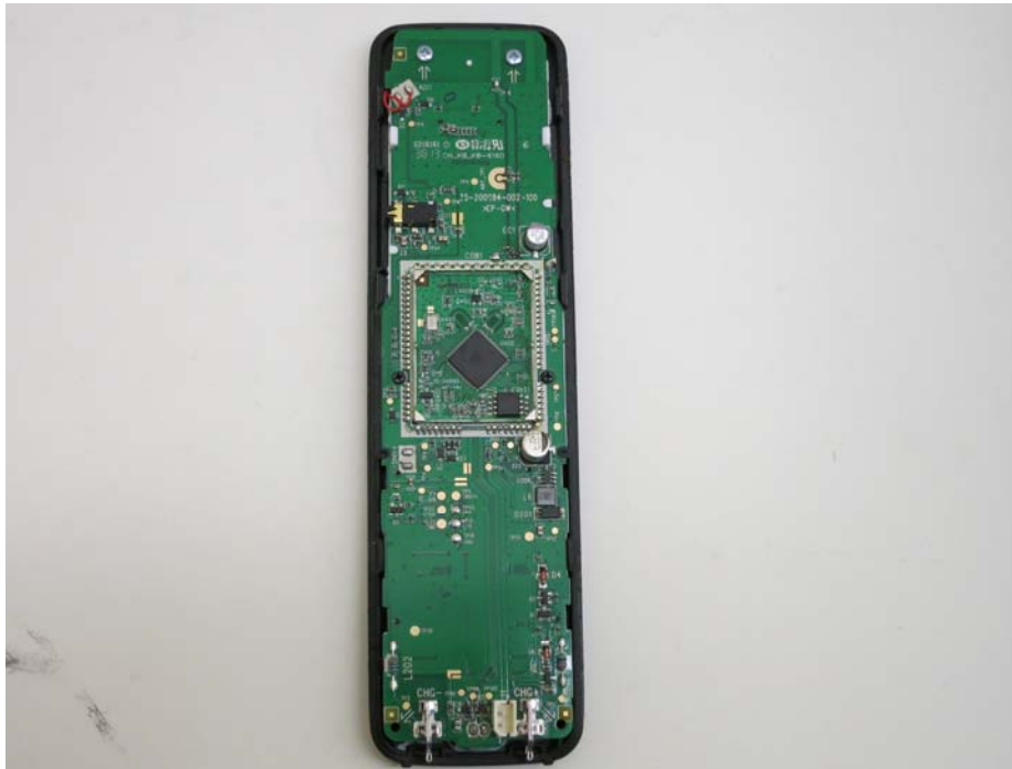
Handset Main PCB comp side (View 1)
