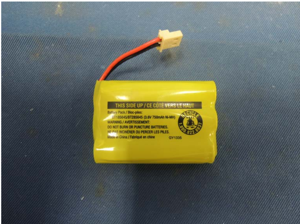
Figure 7 – 3.6V 750mAh GY Ni-MH rechargeable battery pack - Front
