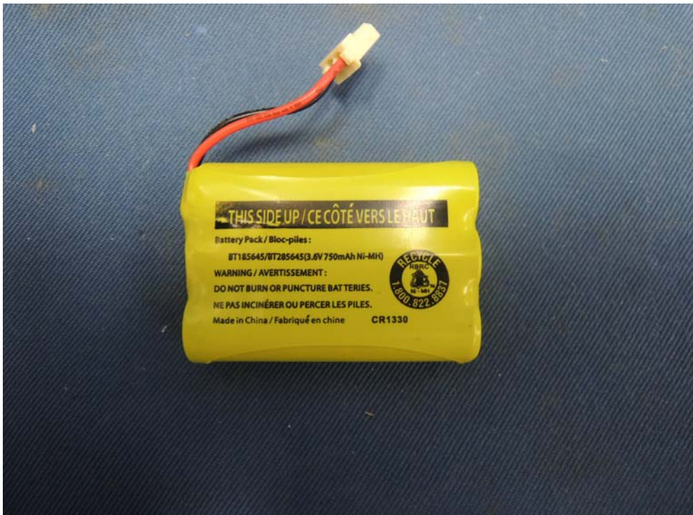
Figure 3 – 3.6V 750mAh CR Ni-MH rechargeable battery pack - Front
