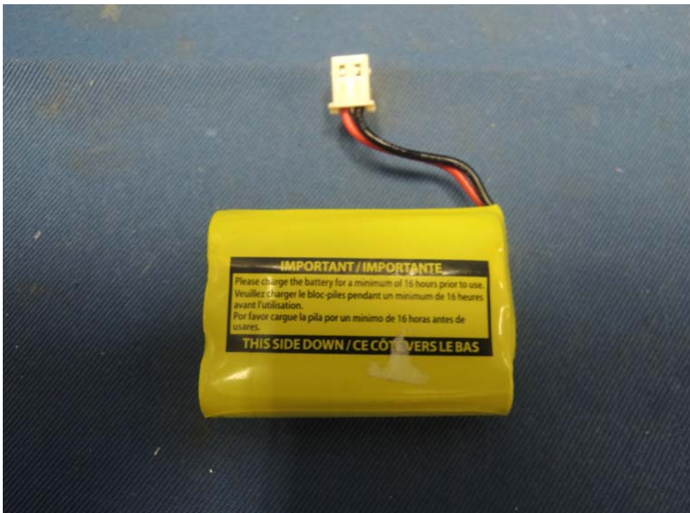
Figure 6 – 3.6V 750mAh GP Ni-MH rechargeable battery pack - Back
