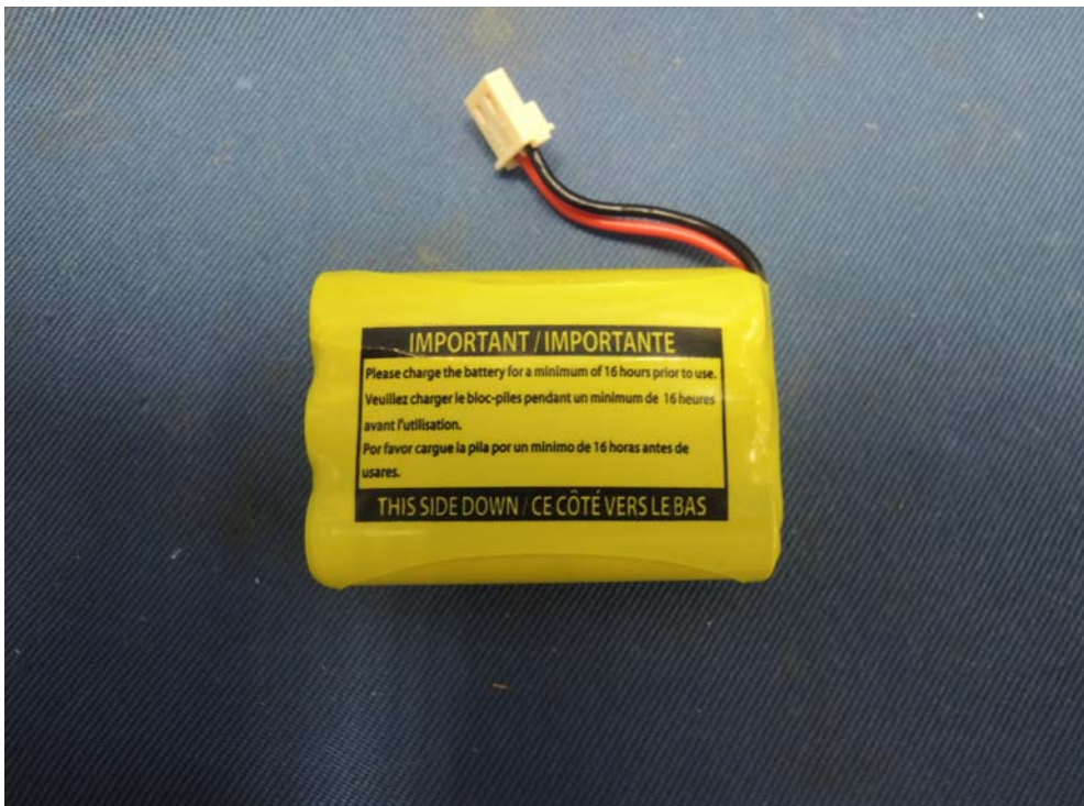
Figure 4 – 3.6V 750mAh CR Ni-MH rechargeable battery pack - Back
