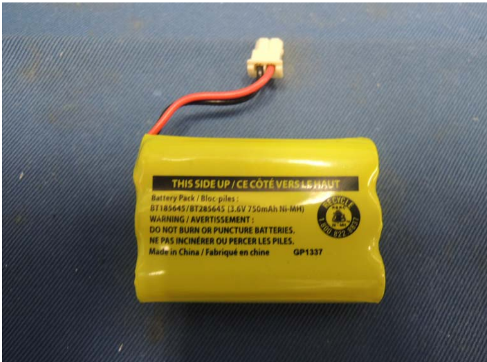
Figure 5 – 3.6V 750mAh GP Ni-MH rechargeable battery pack - Front
