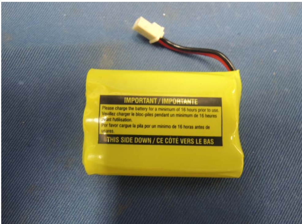
Figure 8 – 3.6V 750mAh GY Ni-MH rechargeable battery pack - Back
