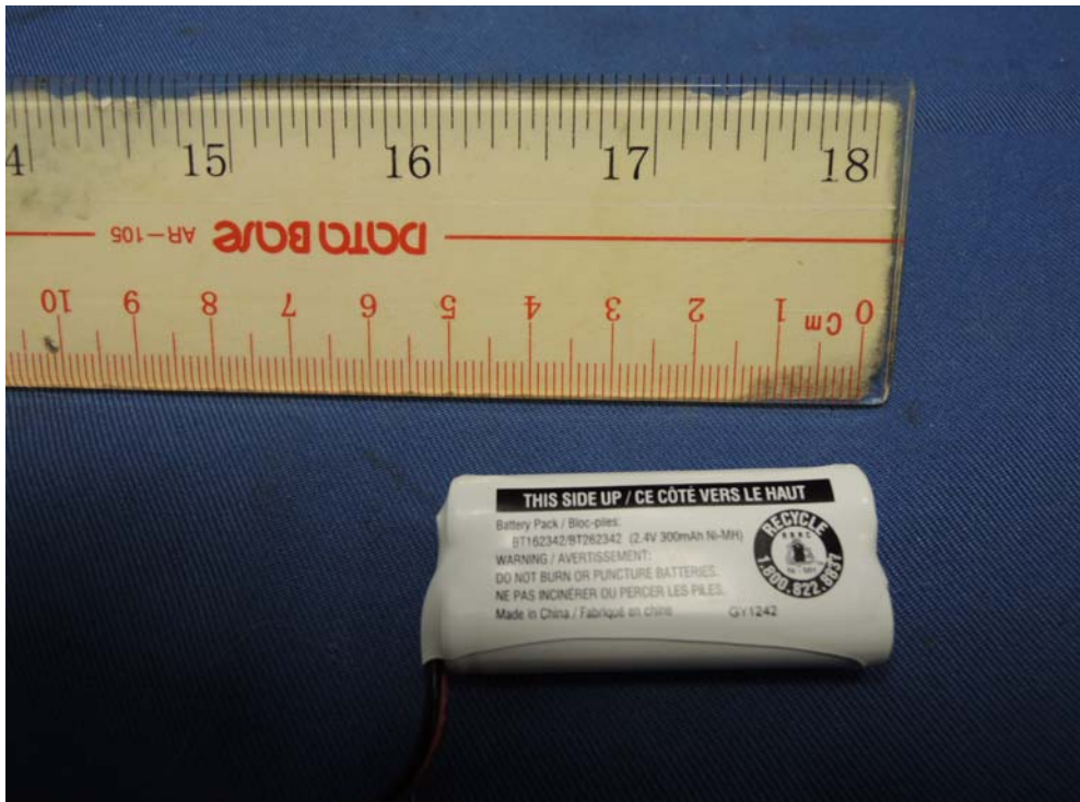
Figure 7 – 300mAh Coslight battery front view
