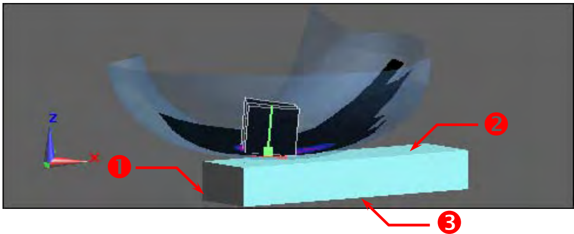
Figure 2. Right Head SAR Test Setup (Cheek)
