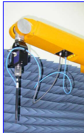
Figure 4. Probe setup on robot
