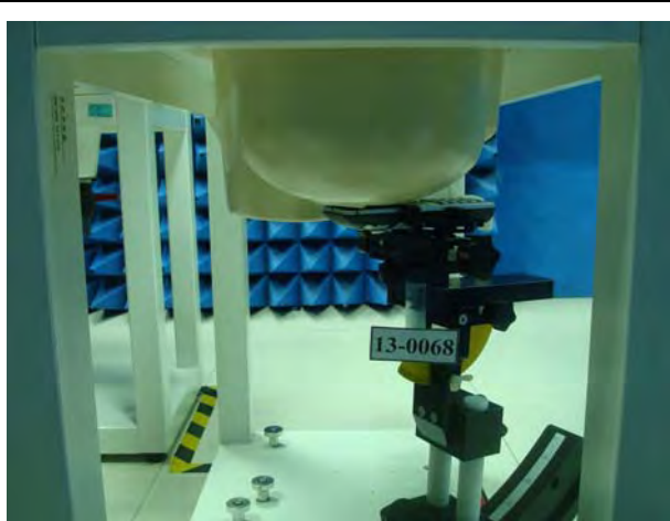
Figure 2. Right Head SAR Test Setup (Cheek)
