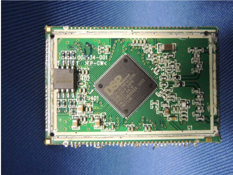
Base Unit DECT Module PCB front side
