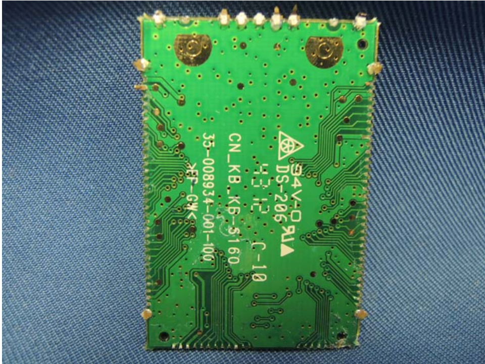
Base Unit DECT Module PCB solder side
