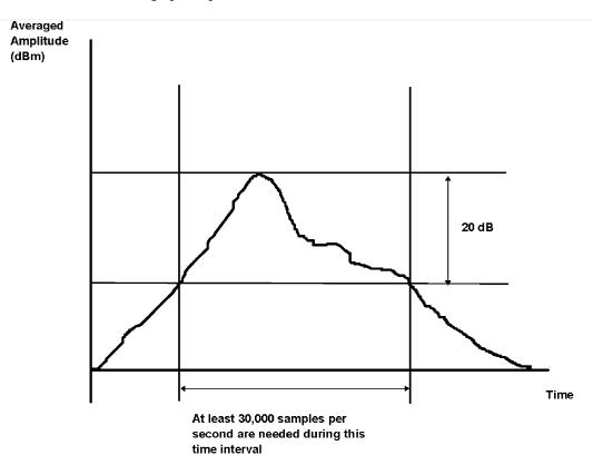
Figure 4—Computed average transient method: Sampling of the averaged power waveform measured with 3 kHz RBW
