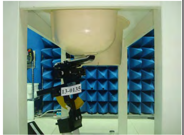
Figure 5. Left Head SAR Test Setup (Tilted)
