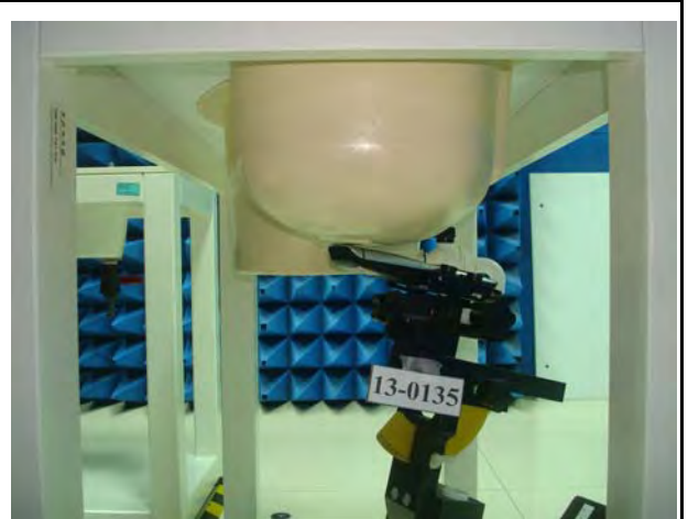
Figure 3. Right Head SAR Test Setup (Tilted)
