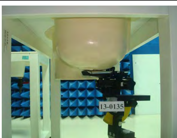
Figure 2. Right Head SAR Test Setup (Cheek)
