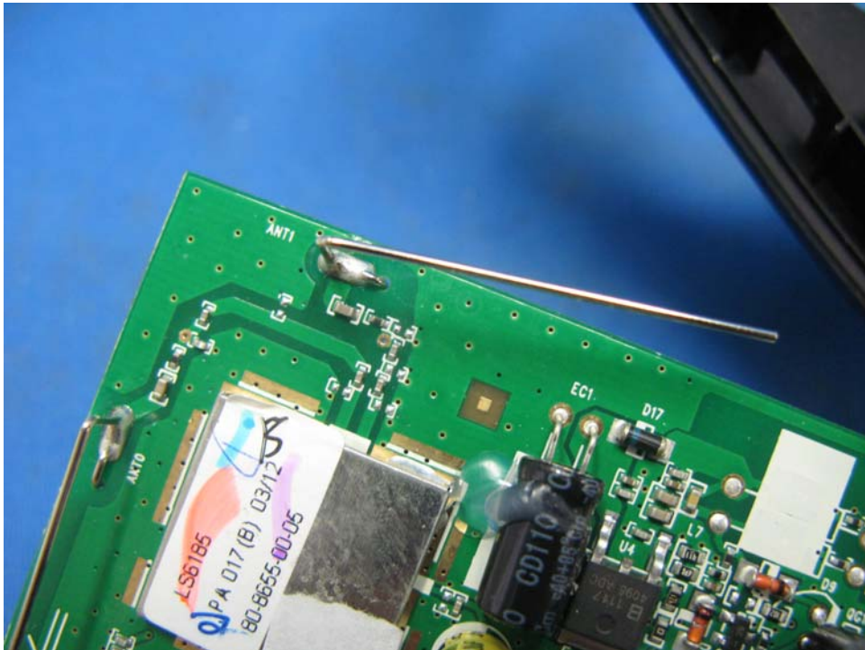
Base Unit DECT Antenna 2
