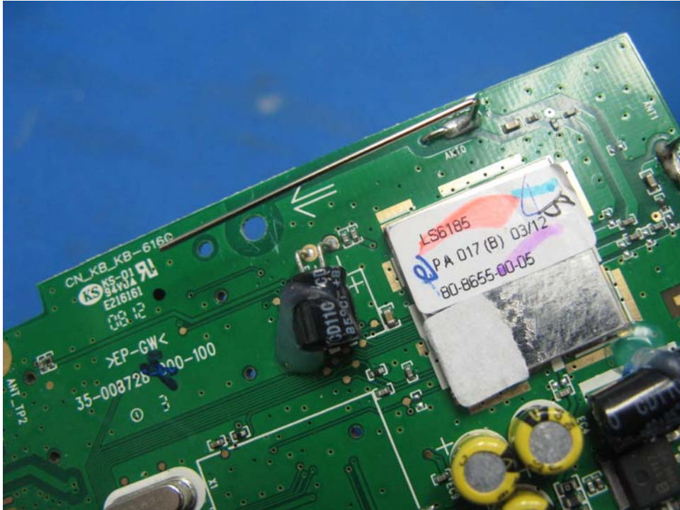
Base Unit DECT Antenna 1
