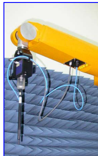
Figure 4. Probe setup on robot
